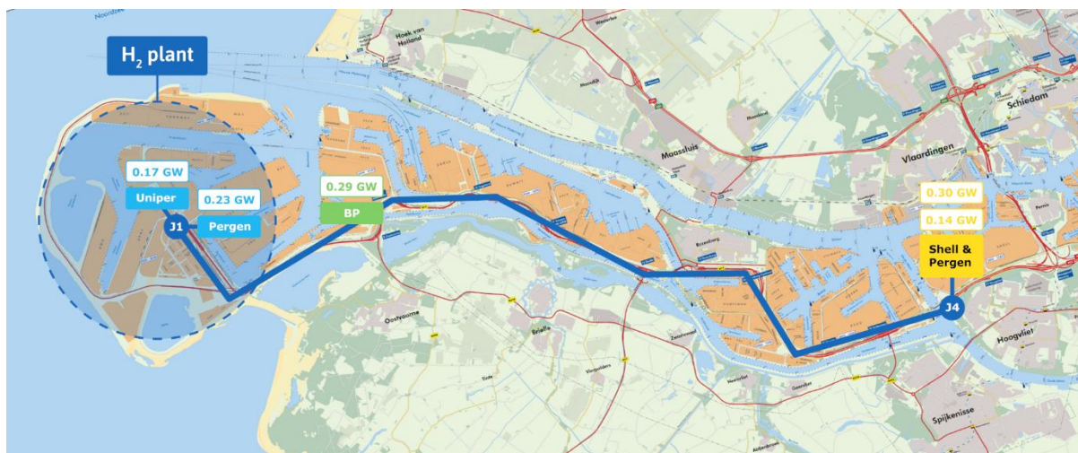
Figure 3.I: Minimum scope (1.1 GW hydrogen demand) overview of the blue hydrogen production and transport infrastructure for the Rotterdam port, including both RFG and NG heating demand from end users. 'J#' are identifiers for junction points where the transmission pipeline splits into smaller lines going directly towards the plants.
