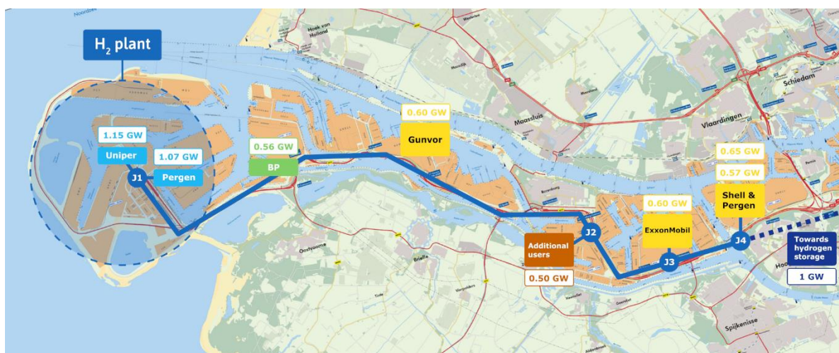
Figure 3.J: Maximum scope (5.2 GW hydrogen demand) overview of the blue hydrogen production and transport infrastructure for the Rotterdam port, including both RFG and NG heating demand from end users. 'J#' are identifiers for junction points where the transmission pipeline splits into smaller lines going directly towards the plants.
